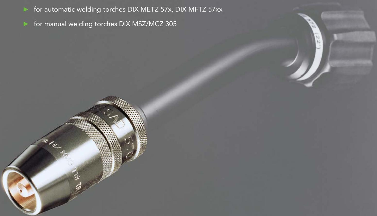
With the dual circuit liquid cooling, the cooling medium flows through the welding torch over the full length in circular channels. The wear parts are cooled separately and thus very effectively; the cooling liquid flows around the gas nozzle.
